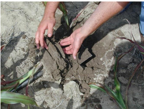
“Platy” soil structure common with soil compaction
